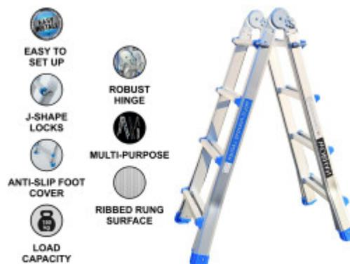
Fully extended length: 413 cm. Step ladder height: 200 cm (at the apex). Rungs: 2 x 7. Distance between rungs: 28 cm. Folded size: 128 cm x 48 cm x 21 cm. Weight: 10.4 kg. Manufactured strictly to EN131 safety standard. Material: Anodized aluminum. Maximum weight: 150 kg. Spaced non-slip ribbed rungs. Safe, simple and convenient locking mechanism ensures ease of working height adjustment.
