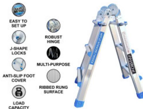
Fully extended length: 303 cm. Step ladder height: 147 cm (at the apex). Rungs: 2 x 5. Distance between rungs: 28 cm. Folded size: 100 cm x 48 cm x 21 cm. Weight: 9.5 kg. Manufactured strictly to EN131 safety standard. Material: Anodized aluminum. Maximum weight: 150 kg. Special non-slip ribbed rungs. Safe, simple and convenient locking mechanism ensures ease of working height adjustment.
